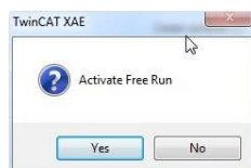
Figure 6-89 EtherCAT integration – Beckhoff TwinCAT | Activate free run message
