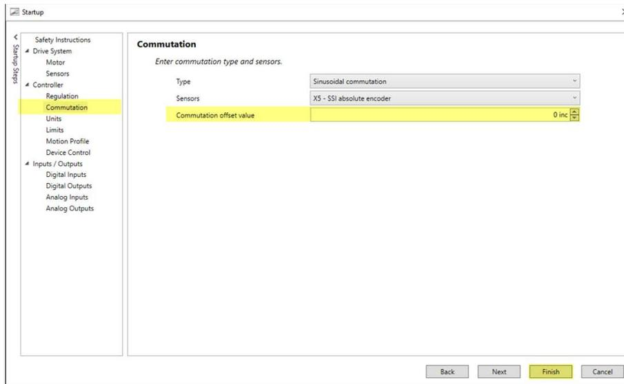
Figure 4-6 Adjustment of SSI & BiSS-C commutation offset value | Set commutation sensor
