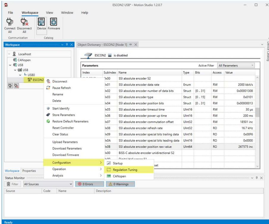
Figure 4-20 Adjustment of SSI & BiSS-C commutation offset value | Identify parameters
