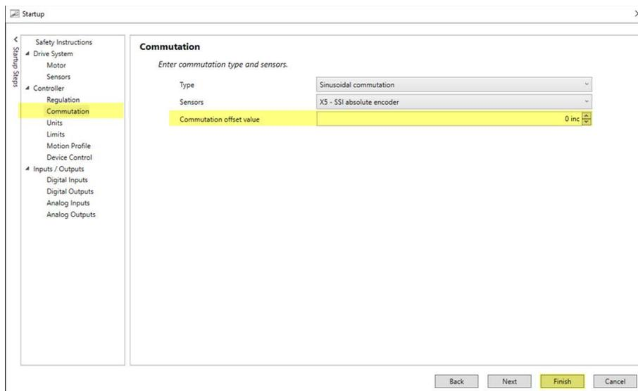
Figure 4-19 Adjustment of SSI & BiSS-C commutation offset value | Set Communication offset value
