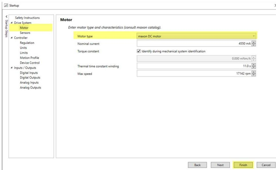
Figure 4-14 Adjustment of SSI & BiSS-C commutation offset value | Select motor type maxon DC motor
