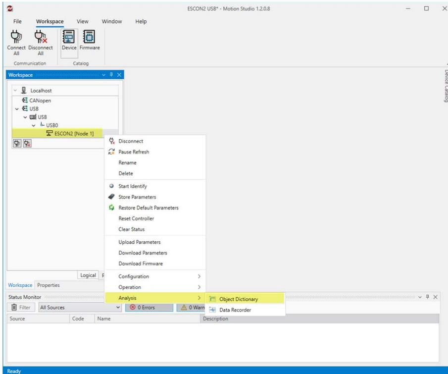
Figure 4-8 Adjustment of SSI & BiSS-C commutation offset value | Open Object Dictionary
