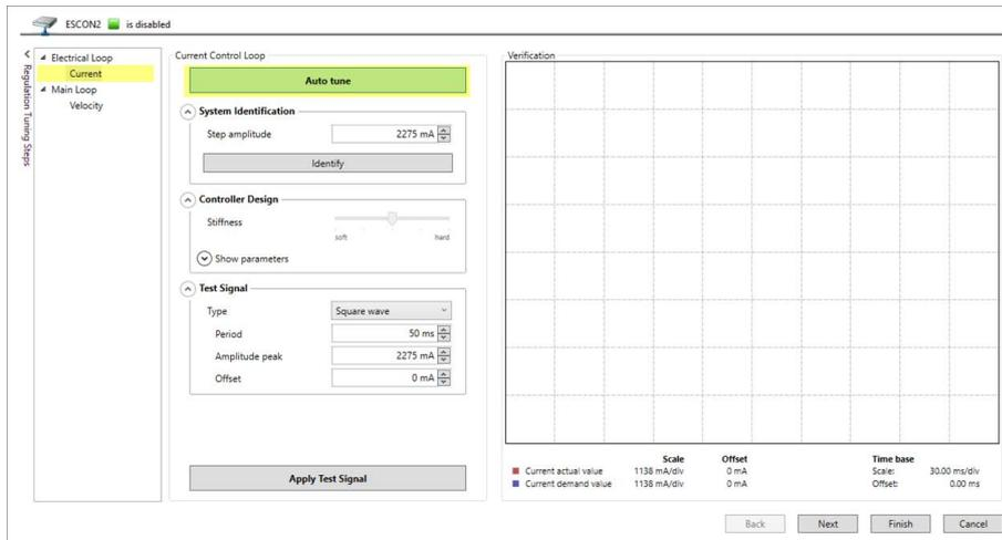
Figure 4-13 Adjustment of SSI & BiSS-C commutation offset value | Auto tuning for current control
