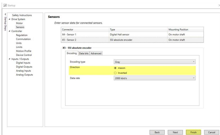
Figure 4-11 Adjustment of SSI & BiSS-C commutation offset value | Toggle direction of rotation
