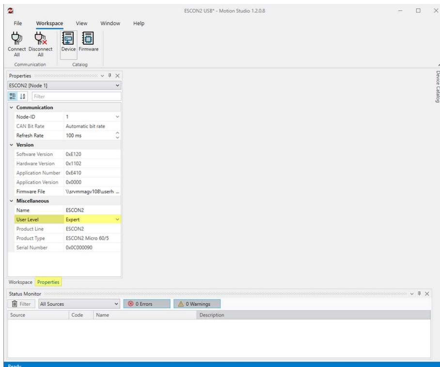
Figure 4-7 Adjustment of SSI & BiSS-C commutation offset value | Switch user level to Expert
