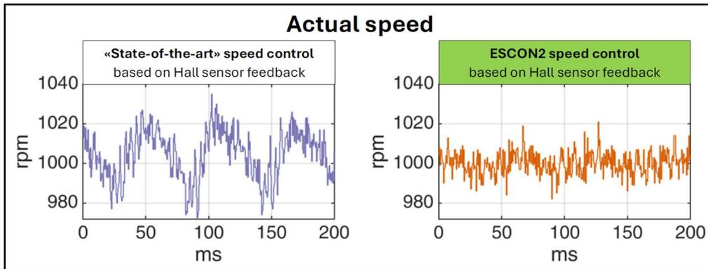
Figure 3-2 Speed stability with Hall sensor feedback
