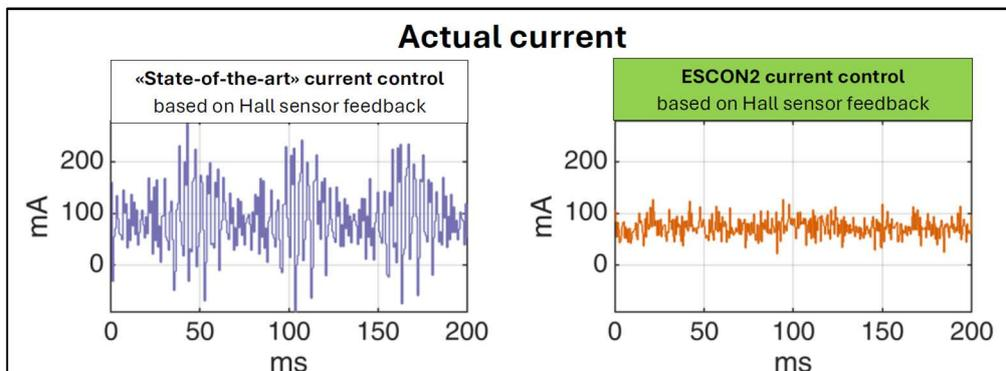
Figure 3-3 Motor current stability with Hall sensor feedback
