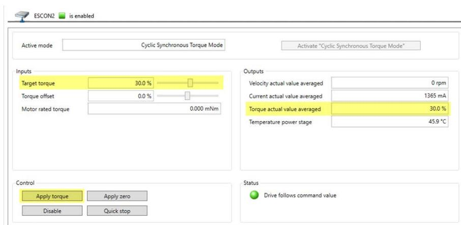
Figure 4-17 Adjustment of SSI & BiSS-C commutation offset value | Apply target torque
