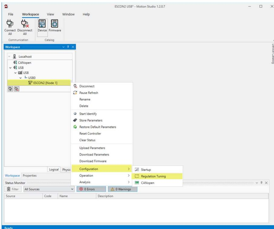
Figure 4-12 Adjustment of SSI & BiSS-C commutation offset value | Regulation Tuning
