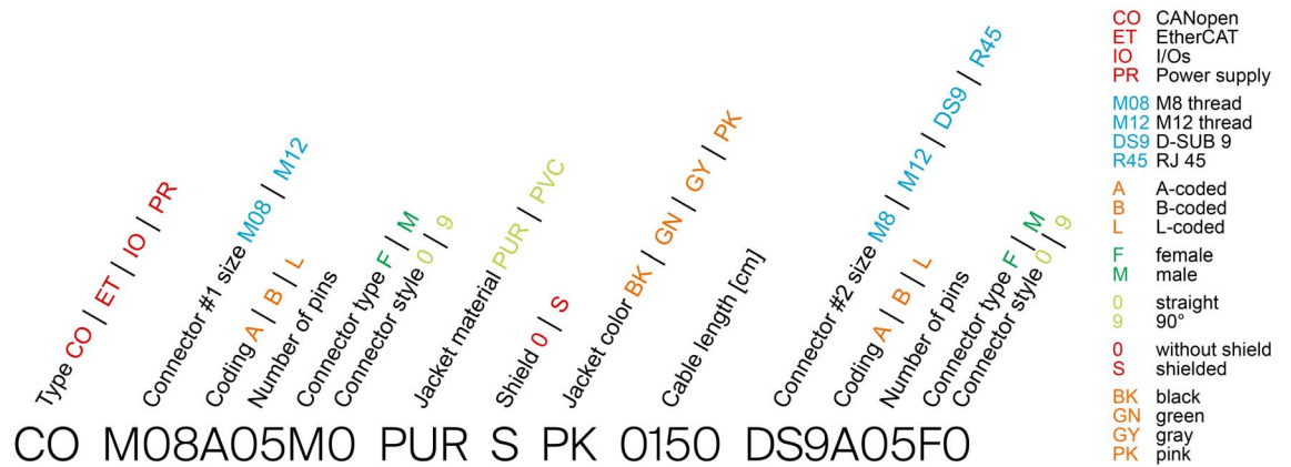
Figure 2-7 Identifiers for cable (examples)
