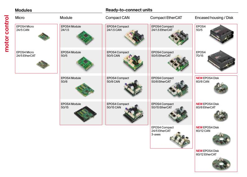
maxon EPOS4 products are small, completely digital, intelligent positioning controllers. Their high power density provides high flexibility for use with brushed DC and brushless EC (BLDC) motors up to approx. 1050 W with various feedback options such as Hall sensors, incremental encoders and absolute encoders, in a variety of drive applications.
