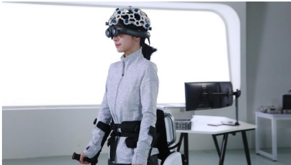
Fourier's exoskeleton, ExoMotus™ X2 combining EEG controlling module. Powerful Actuating Unit – a high-performance motor and gearhead to provide a stronger torque output.
