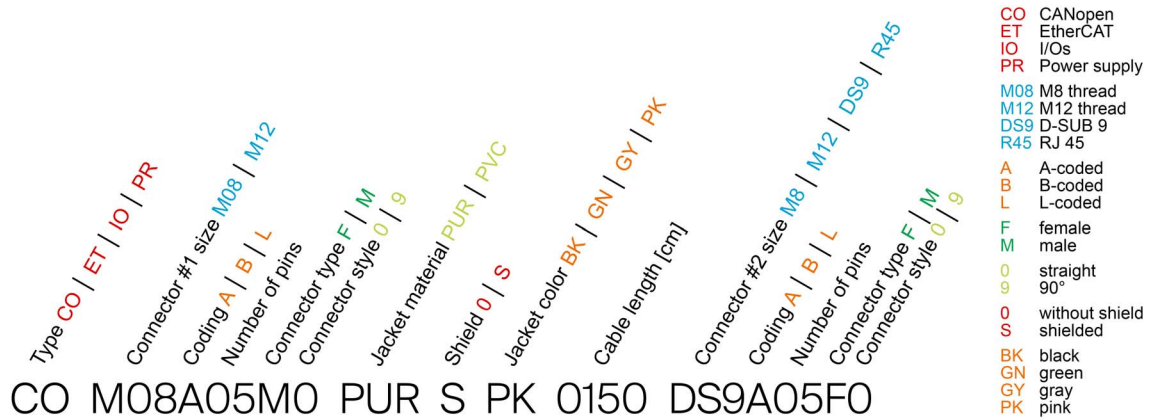
Figure 2-6 Identifiers for cable (examples)
