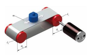
A motor gearhead combination is needed for a conveyor belt application running with a power supply of 24 VDC and 5 A. In a first approximation the conveyor belt is assumed to run continuously at a maximum speed of 0.5 m/s.
