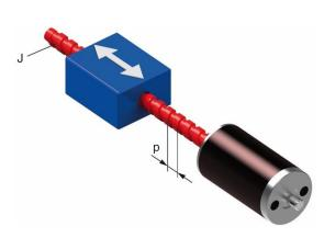
A high precision lead screw with 2mm lead per revolution is used to position back and forth a device in a production plant with short dwell times in between the moves.
