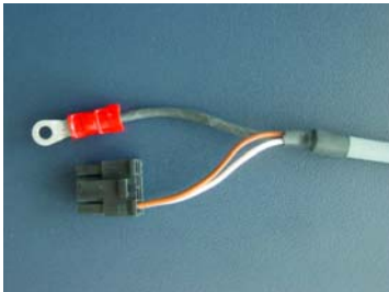
Figure 7: EPOS 24/1 DC motor cable head A
