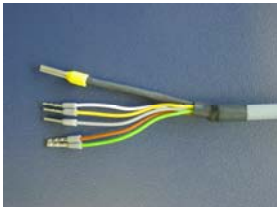
Figure 14: Hall sensor cable head B
