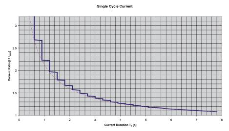
A higher current Imax is permitted for motor acceleration for the period T<sub>a</sub>, after which it is limited to continuous current I cont-
