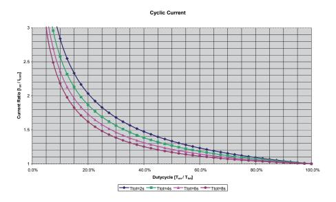
The diagram shows 4 diffrent curves for the total cycle times  $T_{tot} = 2 \text{ s}$ , 4 s, 6 s und 8 s.
