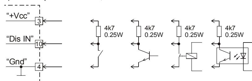
b) Switch open = “Enable”; switch closed = “Disable”
