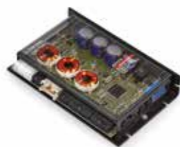
EPOS2 70/10 digital positioning motor controller
