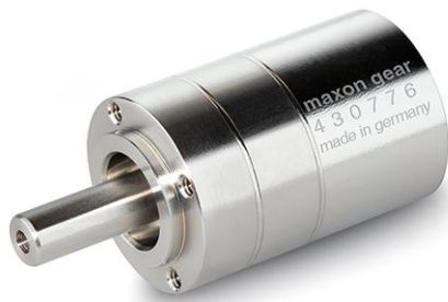
Figure 2: Sterilizable planetary gearhead GP 19 M with a maximum permitted continuous torque of 0.315 Nm and suitable for a motor speed of 40,000 rpm.
