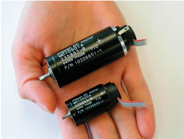
Fig. 2: The RE 25 and RE 20 DC brushed motors from maxon motor have been working on Mars for an entire decade.
