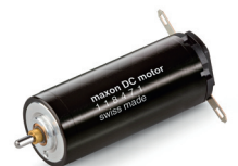
maxon RE 13 Ø 13 mm, precious metal brushes, 2.5 W
