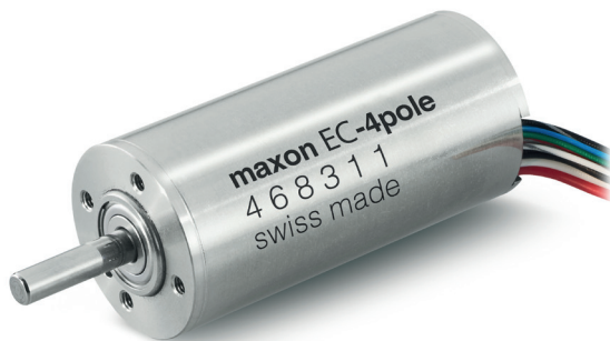
maxon EC-4pole 30 Ø 30 mm, 150 W, brushless
