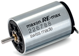
maxon RE-max 29 Ø 29 mm, precious metal brushes, 9 W
