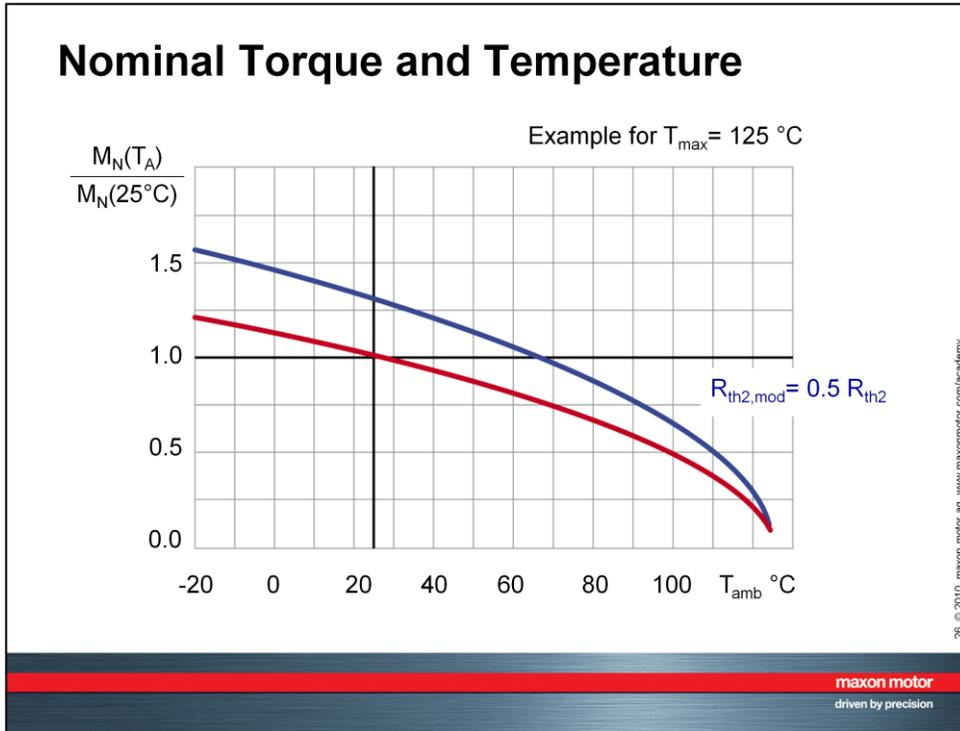
This diagram shows the **influence of the ambient temperature** on the maximal permissible torque (**red curve**). One can see that at temperatures below  $25^\circ$  the permissible torque is higher, while it decreases at higher ambient temperatures.
