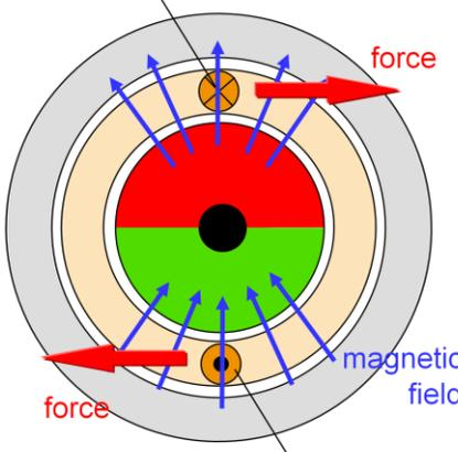
The diagram shows a cross-section of a motor with a central rotor (red and green) and an outer stator (grey). Blue arrows represent the magnetic field, and red arrows represent the force on the rotor segments. Labels indicate current direction towards the brush and flange.
