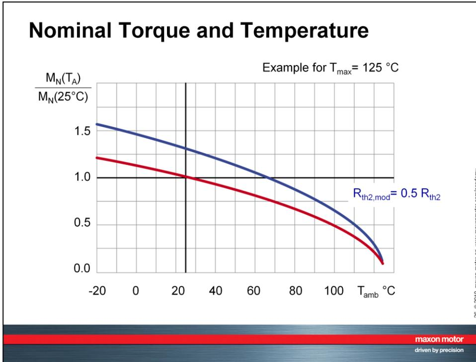
This diagram shows the **influence of the ambient temperature** on the maximal permissible torque (**red curve**). One can see that at temperatures below  $25\text{ °C}$  the permissible torque is higher, while it decreases at higher ambient temperatures.
