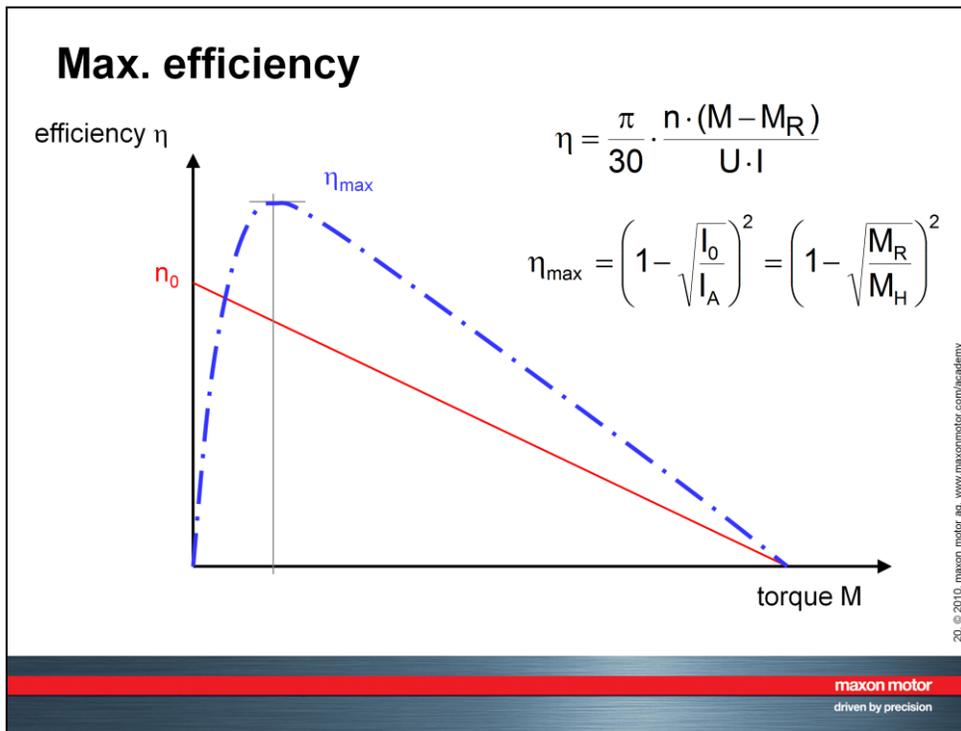
A high **maximum efficiency at nominal voltage** is a nice sales argument. However one should be aware of the fact that this number depends on the applied motor voltage (it increases with increasing voltage) and on the motor torque as shown in the diagram. Running the motor at higher or lower torques results in a lower efficiency.
