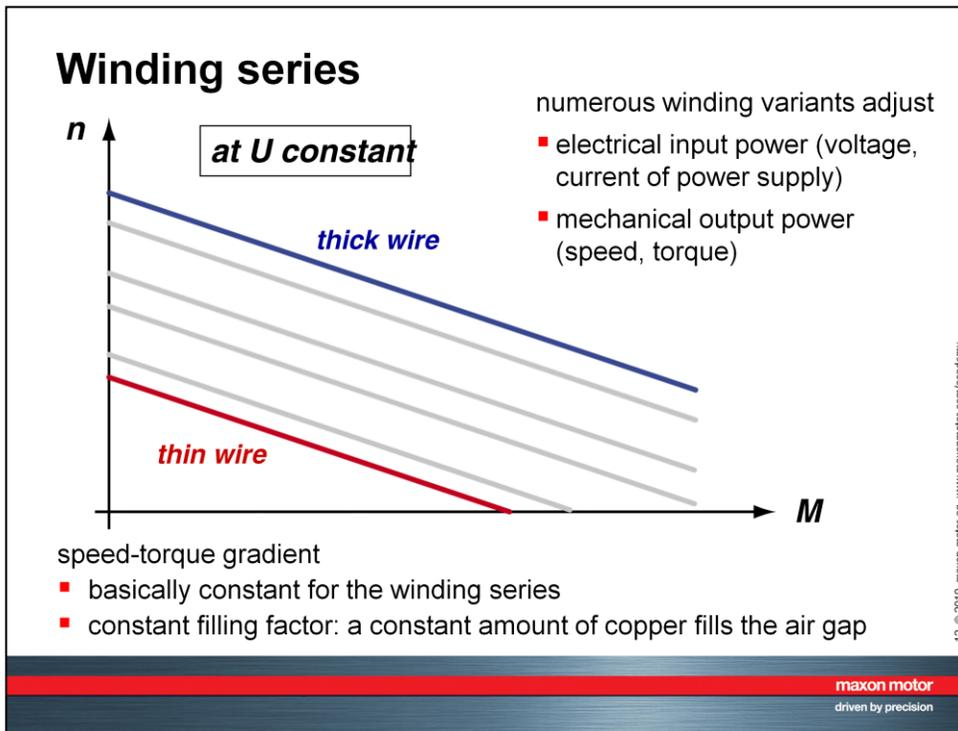
Interestingly, the value of the speed-torque gradient is almost **independent of the winding** used in a particular motor type. Therefore, the speed-torque gradient can be considered a characteristic parameter of the motor type and size and not of the specific winding
