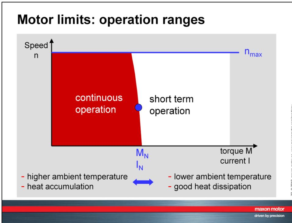
The red area in the operation range diagram represents the **continuous operation range**. Running the motor at speeds and torque in this area will not lead to overheating and a reasonable motor life can be expected.
