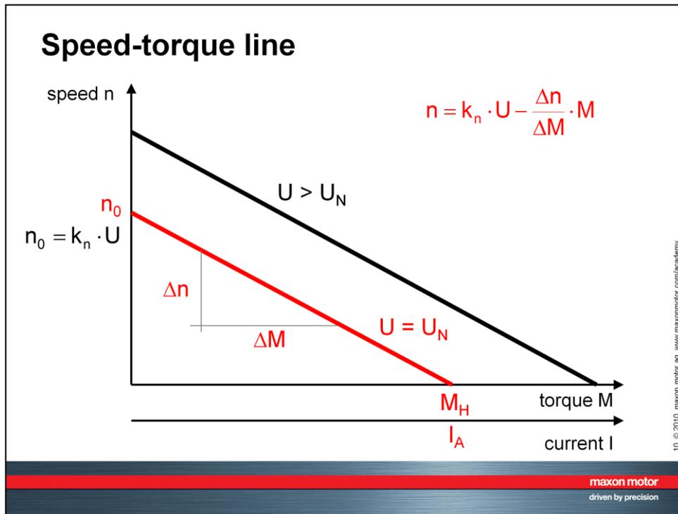
The relationship between speed and torque is the equation of a straight line in our standard representation where the speed is traced as a function of the torque (red line).
