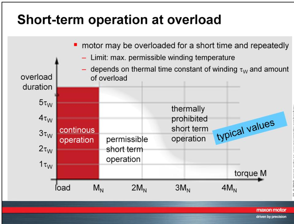
The amount of permissible overload depends on the heating of the thermally weakest part in the motor, i.e. the winding. The winding temperature should remain below the **maximum permissible winding temperature**  $T_{max}$ . The heating of the winding follows an exponential behavior which is characterized by the **thermal time constant of the winding**  $\tau_w$ .
