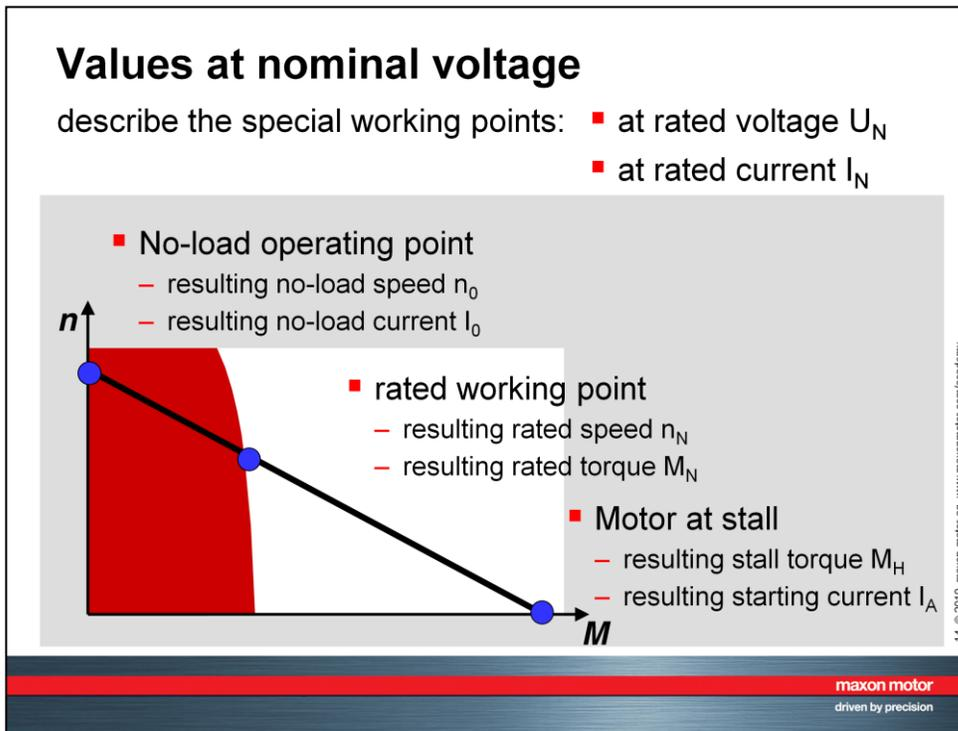
The values at nominal voltage basically reflect three special operating points on the speed-torque line at nominal voltage.
