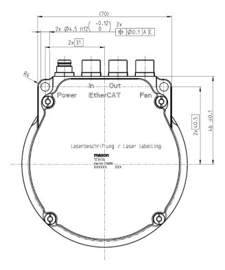
Please note: maxon can offer customized housing geometries, e.g., different thread sizes, hole patterns, attachment points, or heat sinking geometries. Please contact robotics@maxongroup.com
