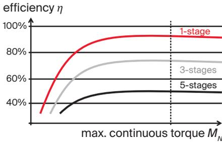
The efficiency specified in the data sheet is a maximum value that applies at loads from approximately 50% of the continuous torque.
