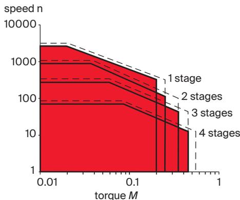
The gearhead losses are stage-dependent (usually about 10% per stage).
