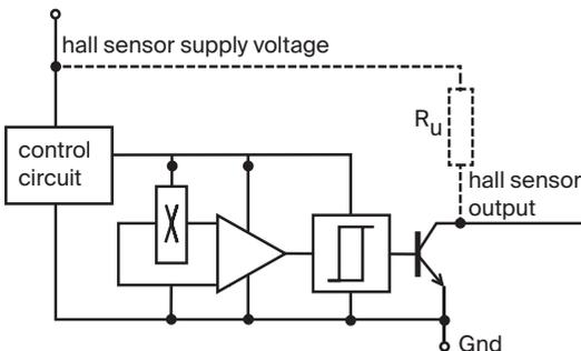
**Hall sensors** usually have an open-collector output without pull-up resistor. Therefore it is integrated into the maxon controllers.
