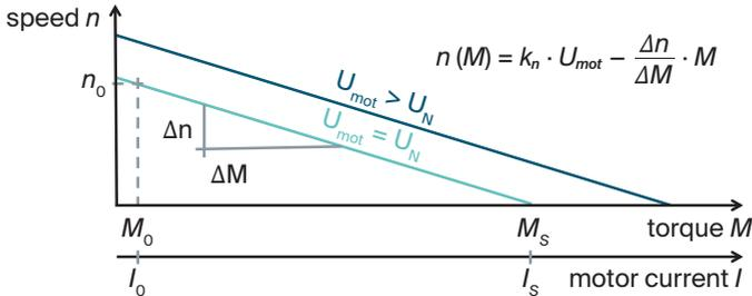
The values of the no load, nominal, and startup operating points specified in the catalog apply at nominal voltage.
