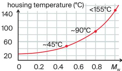
Typical heat build-up in the motor housing in continuous operation ( $T_A = 25^\circ\text{C}$ )
