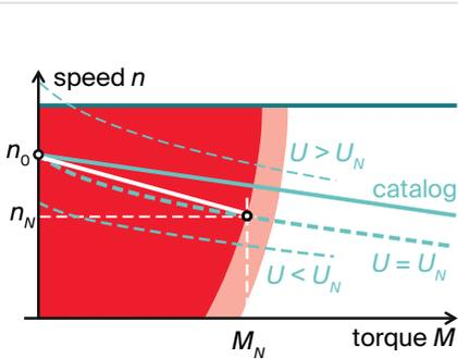
A line drawn between the no load speed and the nominal operating point (white line) can approximate the real gradient in the continuous operating range.
