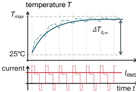
Repetitive work cycles with short durations (typically only a few seconds) can be approximated as continuous operation with the RMS value of the load.
