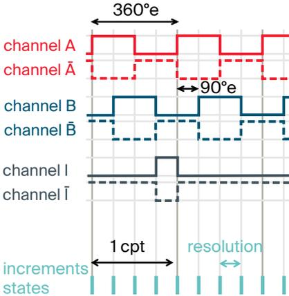
2 channels, A and B, each with  $N$  counts per turn (cpt). If channel A comes before channel B, the direction of rotation is clockwise.
