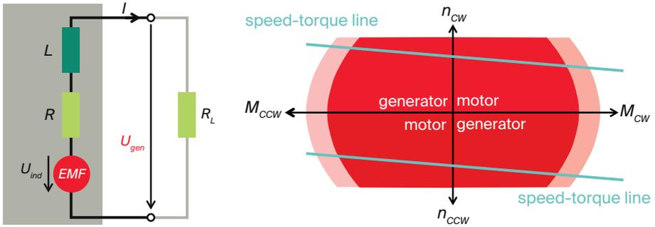
All motor data and limits also apply in generator operation.
