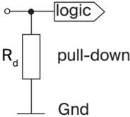
**Pull-down:** (relatively high-impedance) resistor
