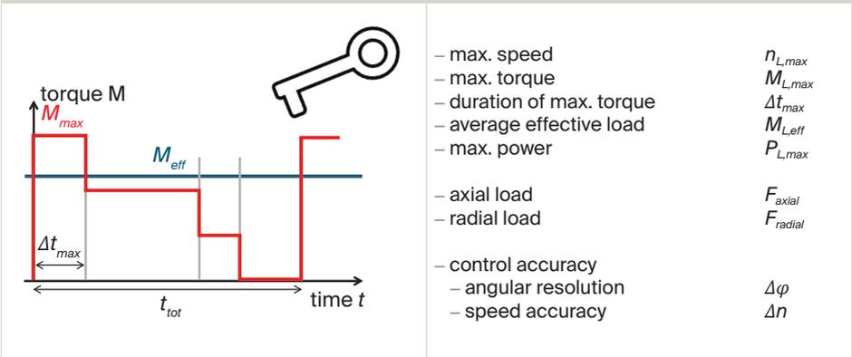
These key load values at the motor level are derived from the calculated input values of the selected gearhead.
