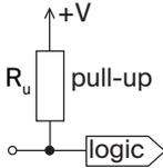
**Pull-up:** (relatively high-impedance) resistor
