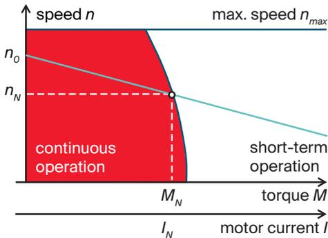
The nominal current  $I_N$  (= max. permissible continuous current) limits the red continuous operating range. Operation at  $I_N$  will heat the winding to the maximum permissible temperature  $T_{max}$ .
