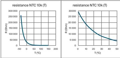
$$T(R) = \frac{1}{\frac{\ln\left(\frac{R}{R_{25}}\right)}{\beta} + \frac{1}{T_{25}}} \text{ [K]}$$
