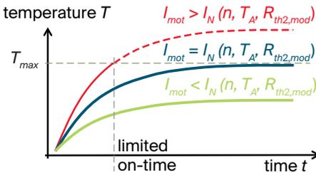
Motor current  $I_{mot} > I_N(n, T_A, R_{th2,mod})$
