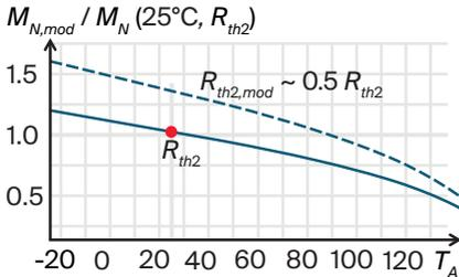
Continuous torque under different
