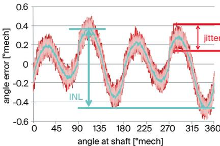
**Jitter:** measurement deviation at the same position across several turns. Frequently caused by axial play.
