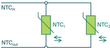
When both NTCs are at the same temperature, the measured resistance  $NTC_{in-out}$  can be used directly to calculate the temperature.
