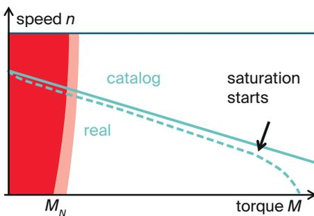
The magnetic saturation of the iron core at high currents leads to a reduction of the torque constant and, consequently, to a decrease of the stall torque  $M_S$ . This deviation is often not taken into account in the data sheet of EC motors with iron core windings.
