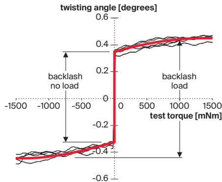
Gear backlash is the turning angle of the gear output shaft which, when the input shaft is blocked, the gear output shaft covers when it is turned from one end position to the opposite position. The end positions depend on the torque applied to the output shaft.
