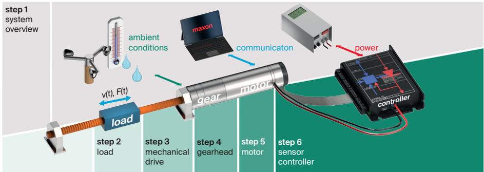
The situation analysis in step 1 considers the drive as a whole together with its environment. The objective is to obtain an overview of the situation, to determine the theoretical feasibility of a solution, and to get a picture of the boundary conditions and special requirements. What type of control is needed, and how will the drive be incorporated into the overall system?
