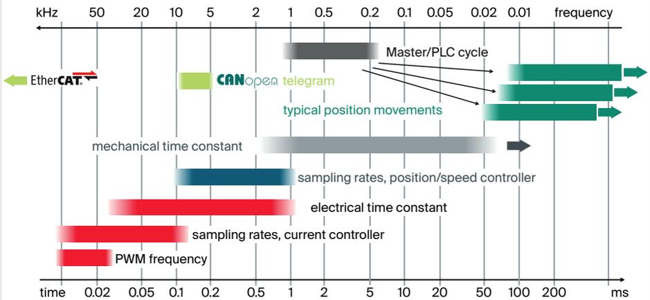
Here the duration of the processes is examined in relation to the mechanical time constant, a measure of how quickly controlled movements can be executed.
