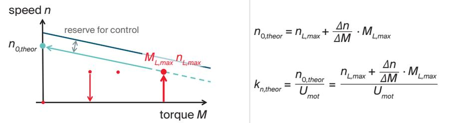
Next, from the data sheet of the selected motor, select the winding with the appropriate speed constant, depending on the operation type.
