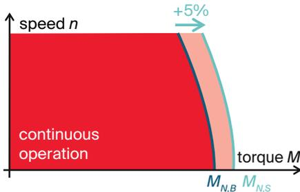
The continuous torque is slightly higher with sinusoidal commutation:
