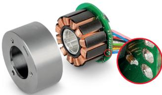
To measure or estimate the winding temperature of a motor, an SMD (surface-mounted device) version of an NTC can be placed on the printed circuit board inside the motor.
