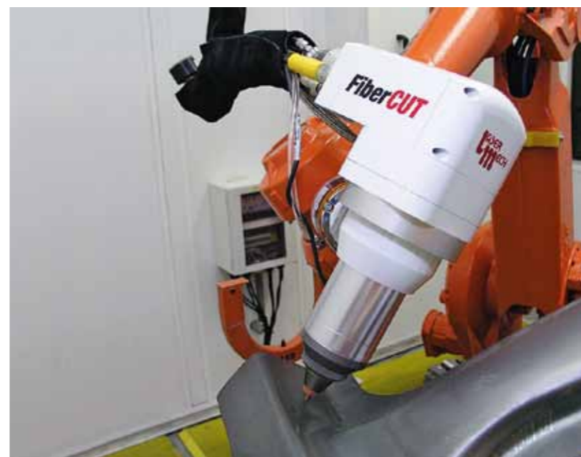
The laser cutting head is primarily used in the automotive industry, for example for cutting chassis beams.
