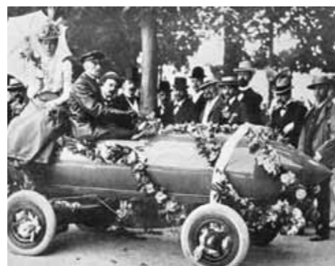
Camille Jenatzy in his electric car that was the first to reach a speed of 100 kilometers per hour.
