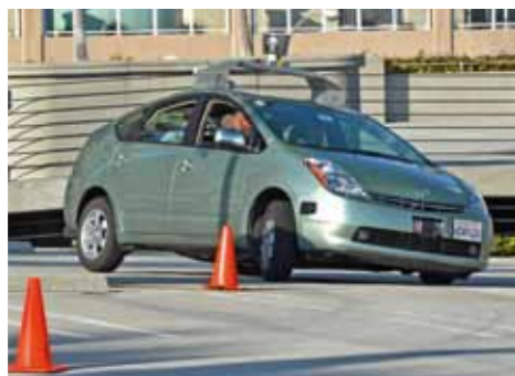
Autonomous cars by Google are equipped with laser, radar, GPS, and cameras.
