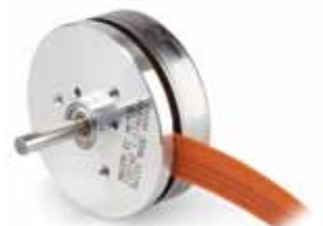
EC 45 flat motors drive the youBot Ø 22 mm, brushless, 100 W, with Hall sensors
