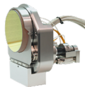
The first prototype of the Field Selector Mechanism (FSM). Two maxon motors are used per FSM unit.
