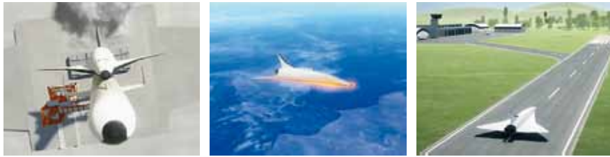
Rocket motors for extreme speeds: After the first thrust, the booster stage separates from the passenger capsule. The plane lands like a conventional passenger aircraft.
