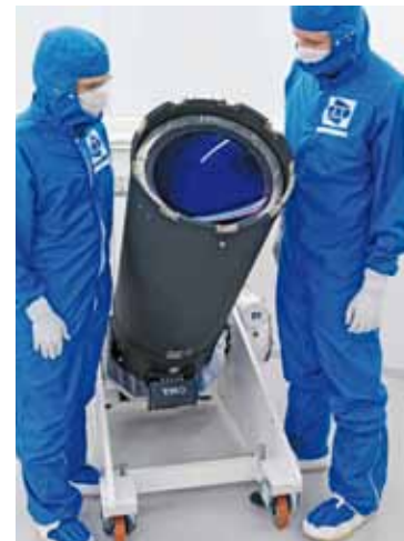
With the Optical Tube Assemblies, laser beams are shot high into the atmosphere to generate artificial stars.
