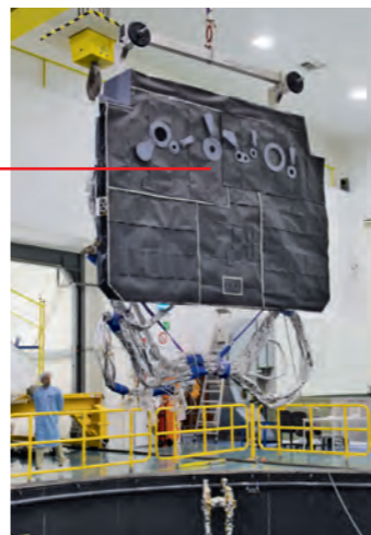
The Solar Orbiter's heat shield has apertures that briefly let the instruments look at the Sun.
