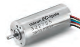
maxon EC-4pole 22 Ø 22 mm, brushless 90 W
