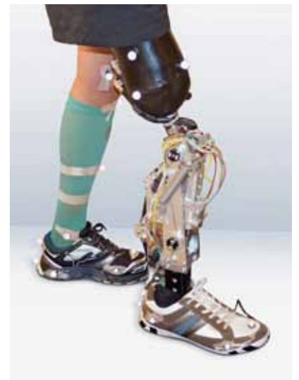
Prosthesis When real power is required, the EC-4pole 30 enters the stage. Its two pole pairs give it an extremely high power density and considerable nominal torque. The motor is also quite robust and resistant to repetitive temporary overload.
