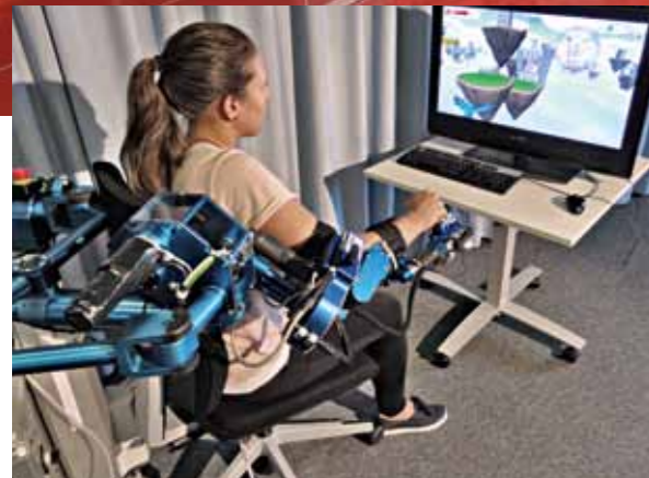
Arm robots Motors of the RE series are used both in the ARMin arm robot and in the children's version, ChARMin. Each motor controls one axis. The two primary axes in the children's version are each driven by one maxon RE-40. Because of the patented ironless winding and the advanced magnet, these motors achieve an efficiency of over 90 percent.
