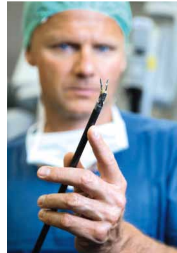
The four arms of the daVinci surgical robot are equipped with various instruments, including a forceps and miniature scissors, as well as a camera.
