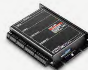
maxon servo controller Esccon 50/5
