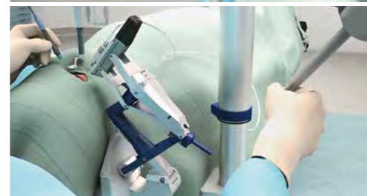
The new robotic system is used in surgery to treat disorders of the retina. Precision with a joystick: When the surgeon moves the joystick by a centimeter, the robotic arm at the extension moves only by a millimeter.
