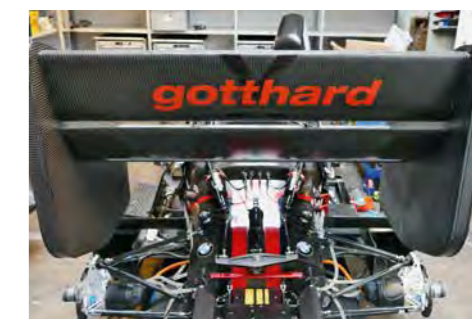
The rear wing reduces the car's drag. It is controlled by maxon motors.
