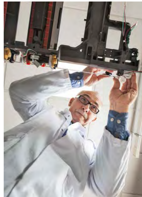
Thierry Bournier is setting the belt tension.
