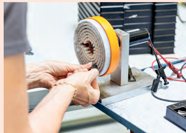
Left: Production manager Walter Kuhn (left) and Andreas Philip, head of the powder injection molding department, standing next to injection molding machines and holding ceramic spindles. Right: Final polish to give the ceramic parts a smooth surface.
