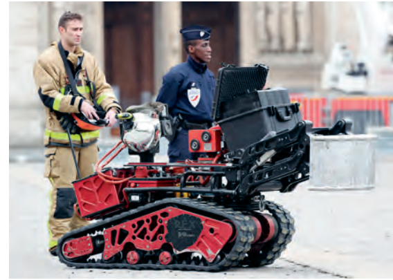
Colossus is about 1.6m long, 78 cm wide and 76 cm tall. It weighs 500kg empty.
