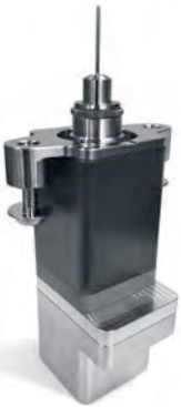
Three of these pinlifters move a wafer in the vacuum chamber.
