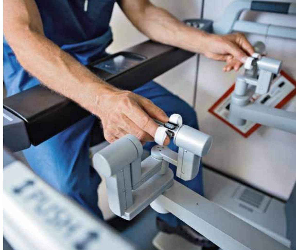
The daVinci surgical robot is controlled manually using two joysticks.
